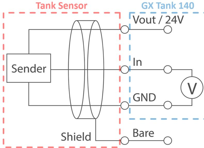
The table below shows the wiring connections in a tabular format, including the tank sensor connection names and common wiring colours.
