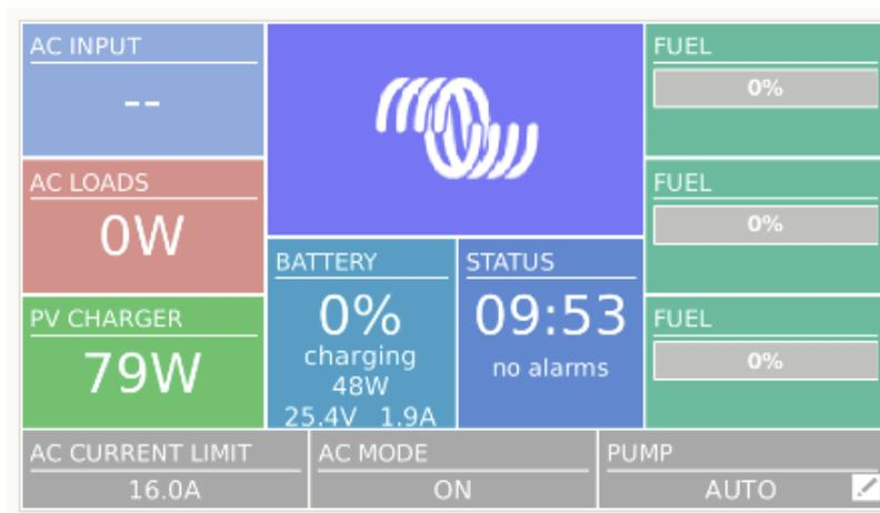
It is also possible to change the pump 'Mode' (between 'Auto', 'On' and 'Off') directly via the 'Boat and motorhome overview' page.
